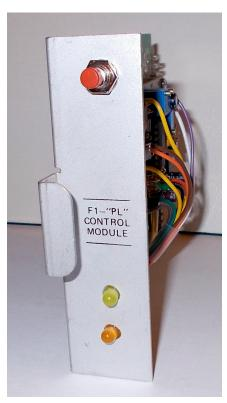
Here's the finished cor board, installed on the card, aligned, tested and ready for deployment (in service) in the Spectra-tac receiver unit. For maintenance tracking each card is serialized. This particular card needed the monitor button added. Also, the timer and AF settings are indicated to be set.
